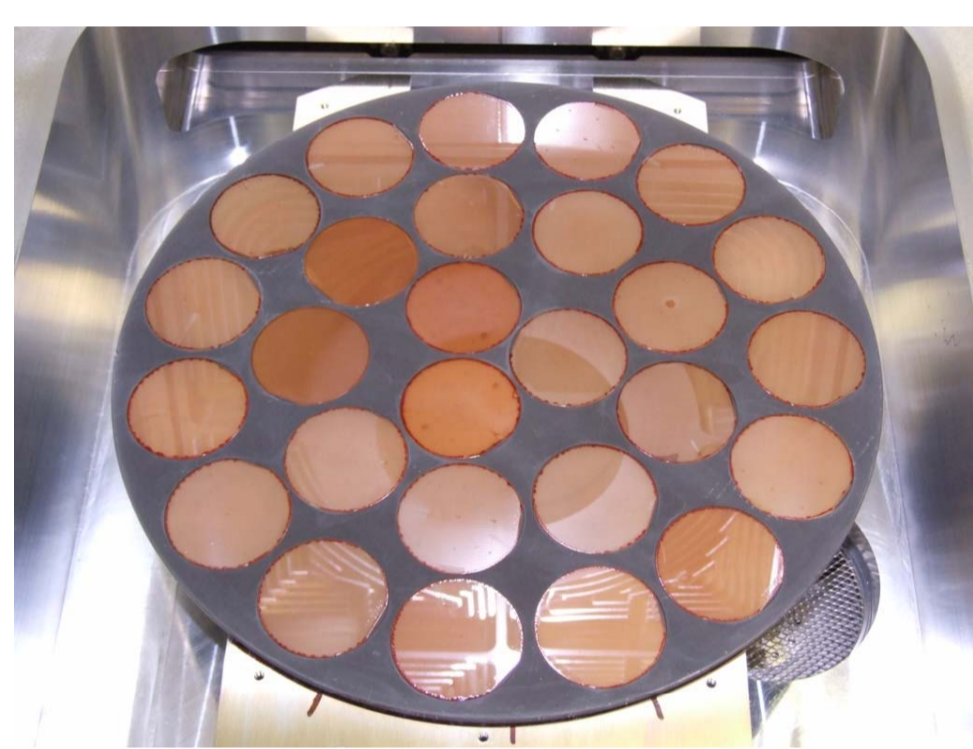
Figure 1 27x2 inch GaN wafer were placed on a SiC carrier-plate for process.
