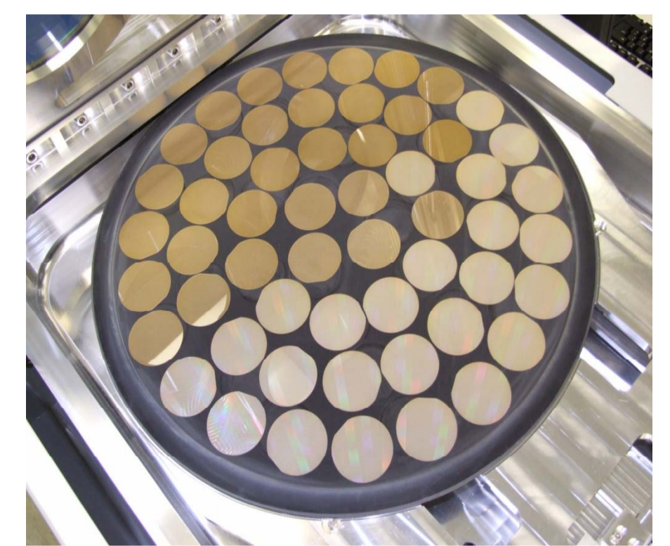
Figure 10 (right), 55x2 inch GaN wafer were placed on a SiC carrier-plate for process.
