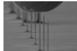
Tungsten probe contacting a 60 nanometer diameter silicon pillars, 2.5 microns tall. Etched using an alumina etch mask and Pseudo Bosch etch in an Oxford Instruments Plasmalab System100 ICP-RIE 380.
