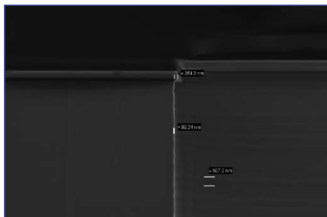
Sub-100nm sidewall roughness for Bosch DSE
