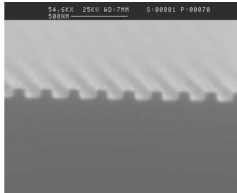
Figure 8 CH_4/H_2 grating etch
