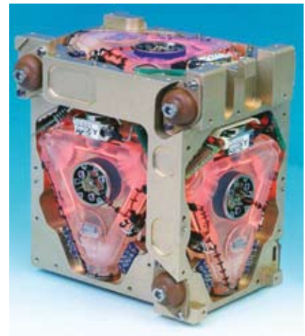
Low loss mirrors produced by Ion Beam sputter deposition are incorporated into this inertia sensor assembly which incorporates three ring laser gyroscopes. Image courtesy of Marconi Electric Systems
