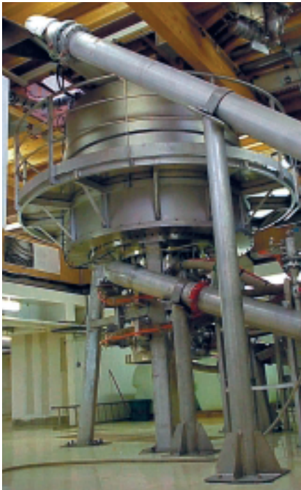
Figure 2 The fully assembled cryostat
