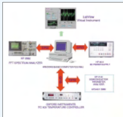
Fig. 1: Measurement and control instruments interfaced via GPIB bus to a virtual panel.
