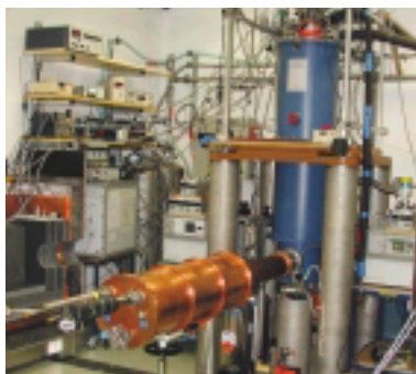
Figure 1. The copper cold box connected to the Oxford Instruments dilution refrigerator Kelvinox-300.
