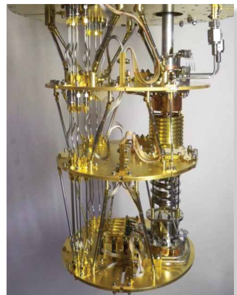
Triton200 with 10 x high frequency coax, 2 x fibre optics, 10 x flexible coax, 96 D.C leads. Temperature achieved < 10mk.
