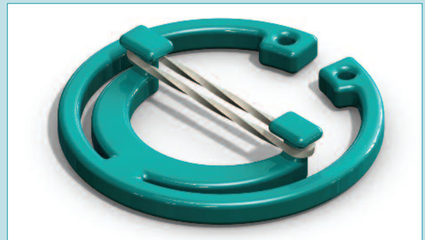
a. Retaining band holds a tablet in place, used in early experiments.
