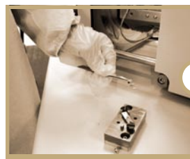
FIG.4 - Transfer of the FIB cassette with a lift-out sample to the mechanical conversion anvil.
