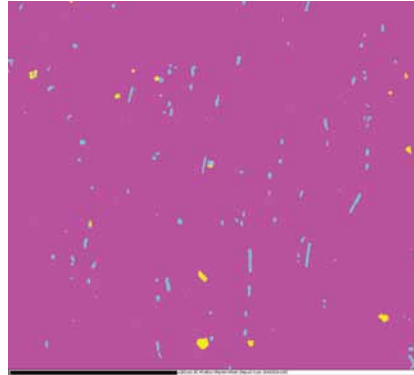
Figure 3b: Low magnification EBSD phase maps (fuchsia=matrix, aqua= M_{23}C_6 and yellow=AlN).
