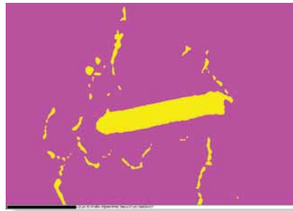
Figure 5b: Phase map (where fuchsia=matrix and yellow= carbide phase).
