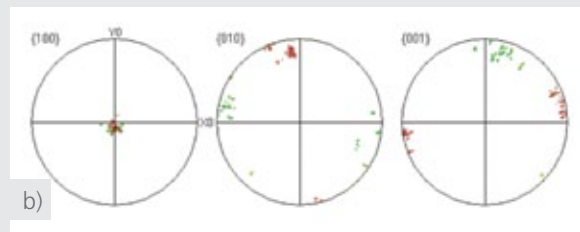
Figure 3. a) 8 kV High resolution EBSD IPF X plus pattern quality map from the image in Figure 1b and b) set of scattered pole figures from the map in 3a.
