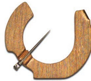
The Short-Cut™ makes triple-compatible atom probe/TEM/tomography samples
