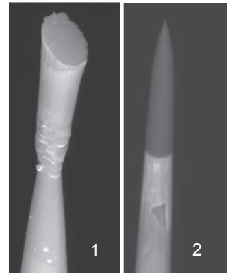
Sample on probe tip after release (1) & final shaping (2)
