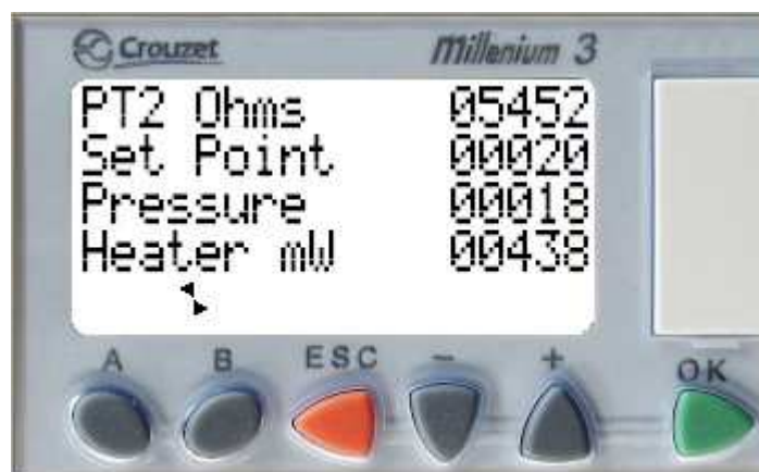
Fig 6-8 Display showing the measured resistance of the Allen-Bradley temperature sensor. The rest of the display is the same as normal mode
