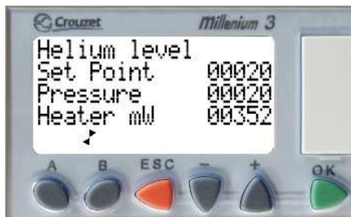
Fig 6-2 The display after selecting the Helium level item from the options menu
