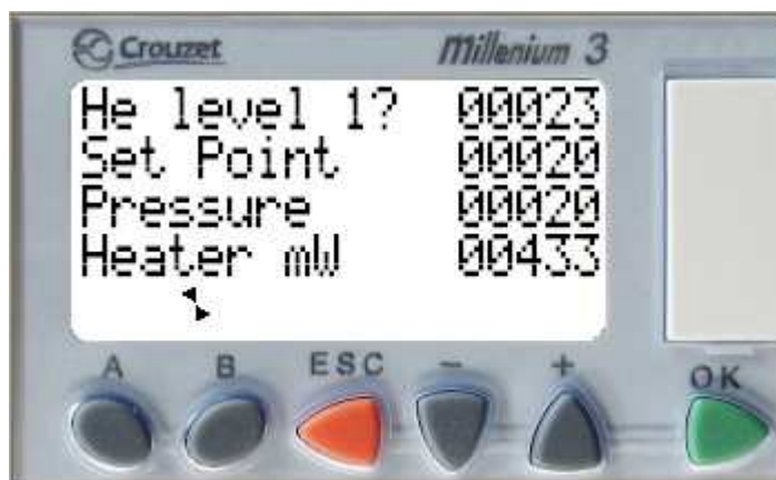
Fig 6-11 Display for the "Set He level 1" mode. The rest of the display is the same as normal mode
