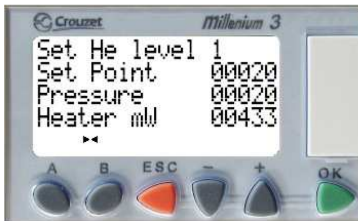
Fig 6-10 Display to select "Set He level 1" mode. The rest of the display is the same as normal mode
