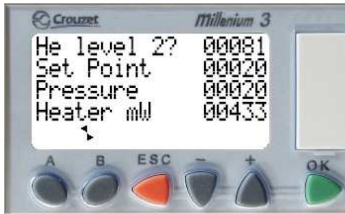
Fig 6-13 Display for the "Set He level 2" mode. The rest of the display is the same as normal mode
