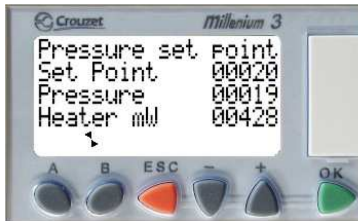
Fig 6-6 Display for pressure set-point adjustment mode.
