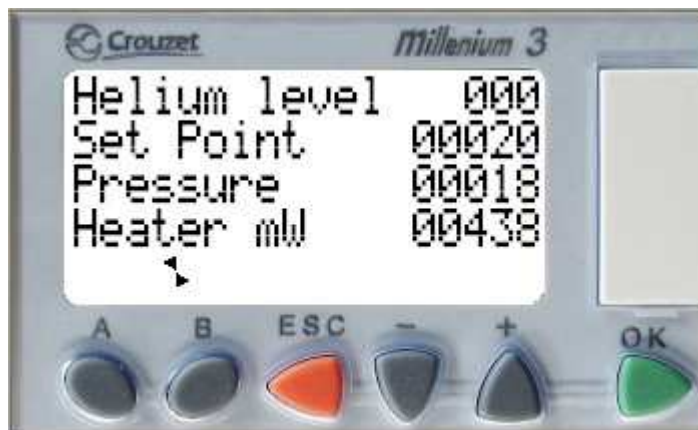
Fig 6-3 Display showing Helium level (in this case the Helium level is 0%)
