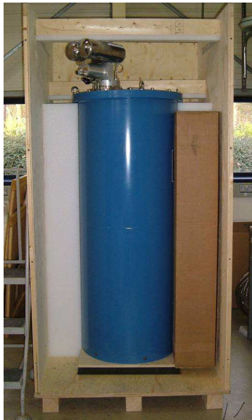
Figure 4 - Cryostat in box with top and side removed
