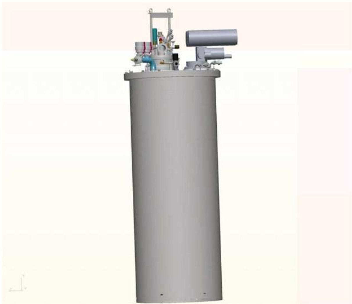
Figure 1 Illustration of Integra AC system showing the Cryostat, pulse tube and an example of an insert
