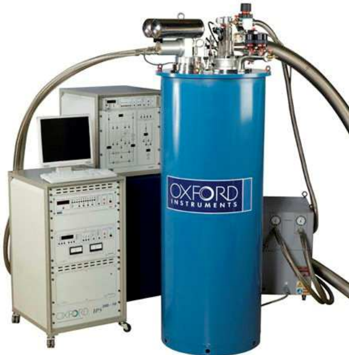
Figure 3 Illustration of a typical Integra AC system showing the cryostat, pulse tube refrigerator, Compressor and refrigerator unit
