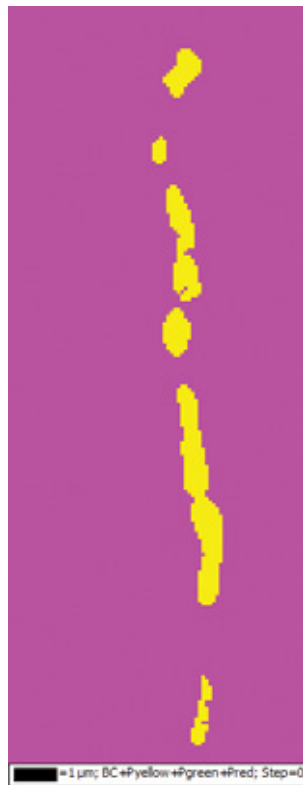
Figure 4b: Phase map fuchsia=matrix and yellow=carbide phase.
