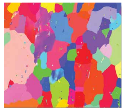
Figure 3i: IPF X coloured map for all the phases.
