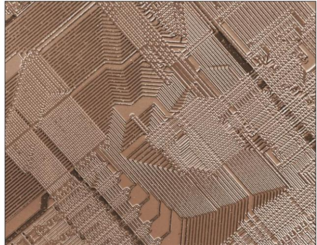
This application focuses on the significance of grain and boundary characteristics in 500 nm wide copper lines produced by the Damascene process.
