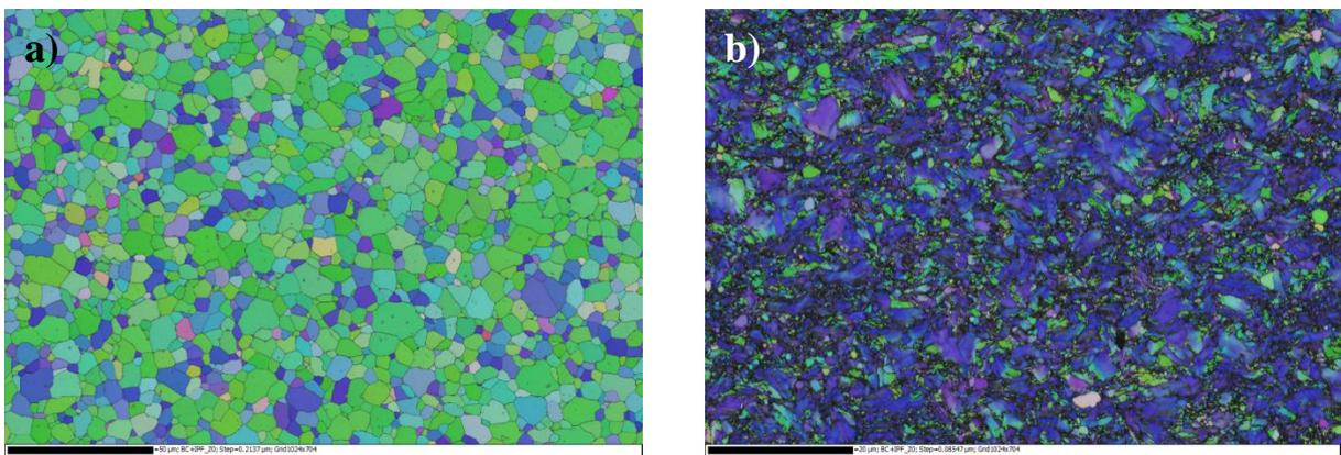
Figure 3. EBSD IPF Z coloured maps a) starting tube and b) after reduction.
